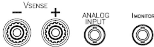
Fig 2-7 34000E Series I/O Connection
