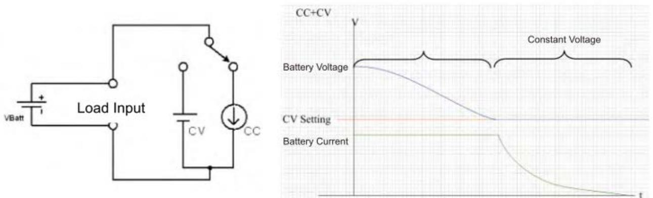
Fig 5-8 CC+CV mode operation application
