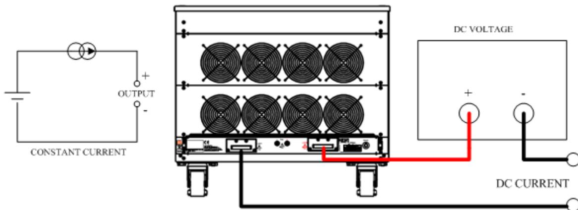
Fig 5-10 constant current source connection
