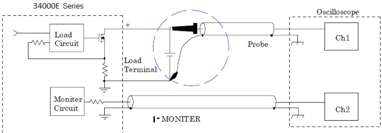
Fig 3-4 (Correct) Connections to an oscilloscope
