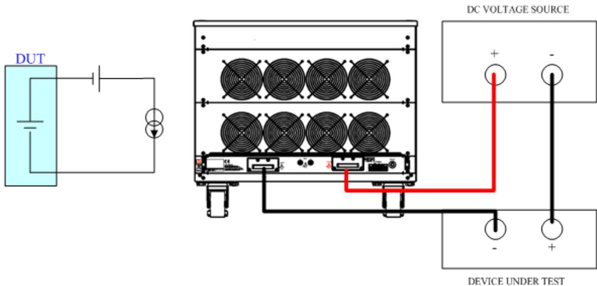
Fig 5-11 Zero-Volt loading connection
