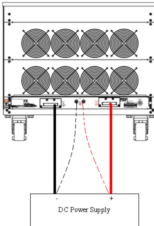
Fig 5-2 Remote voltage sense connections
