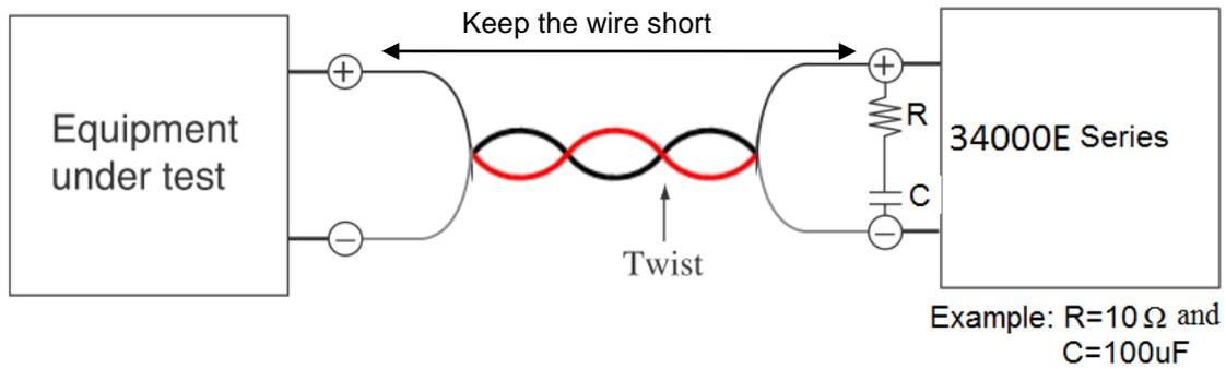
Fig 2-10 Length of wiring
