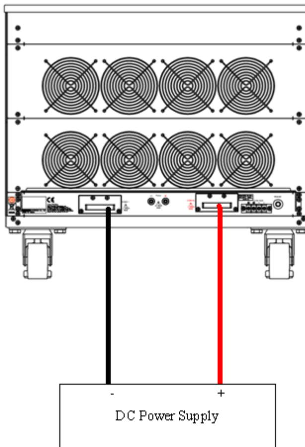
Fig 5-1 Local voltage sense connections
