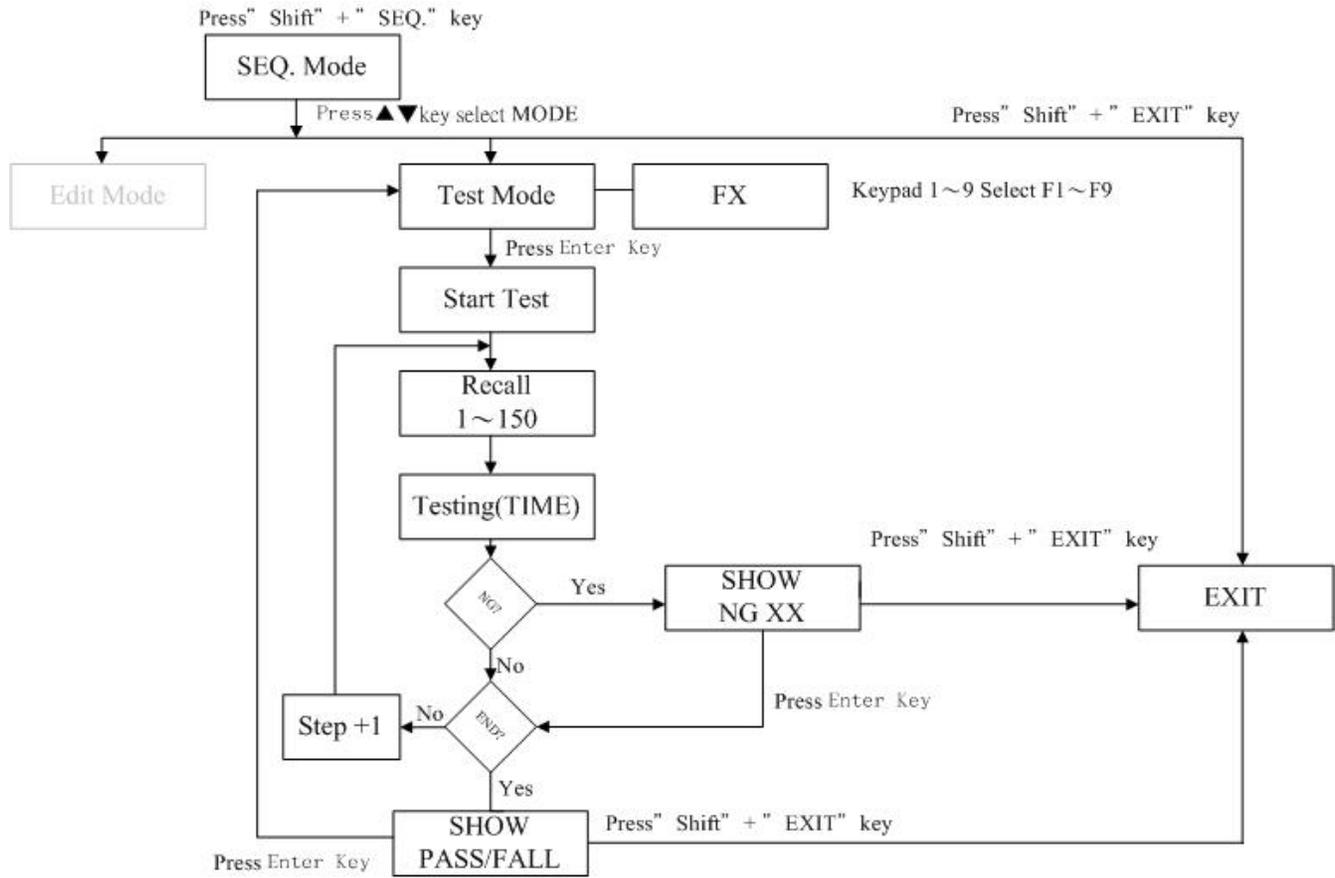
Fig 3-8 TEST MODE OPERATION FLOW-CHA
