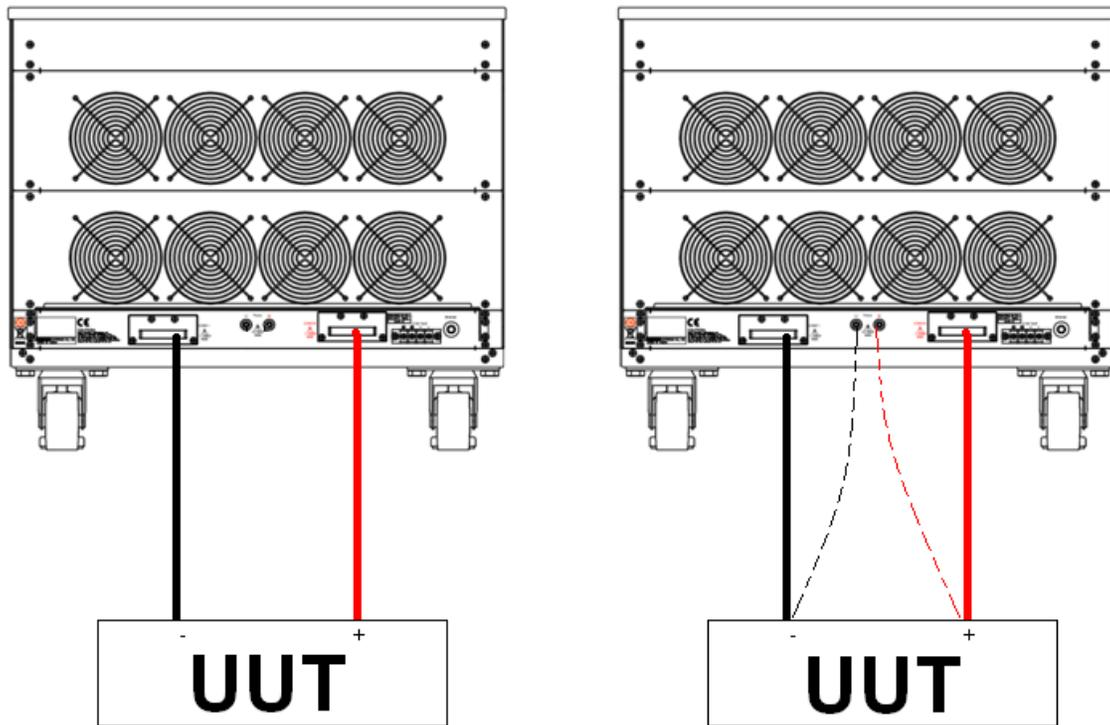
Fig 3-2 typical connection of 34000E series load module
