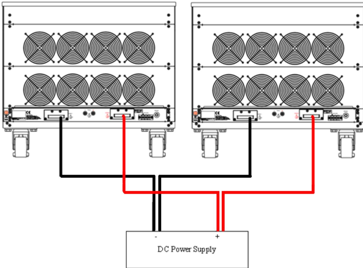
Fig 5-12 34000E series load parallel operation
