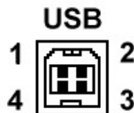
Figure 3-2: USB Connector pin orientation
